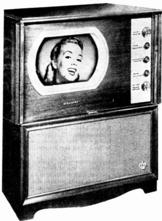
The Air King — first dual-color television receiver manufactured after the FCC approved the CBS color-television system. The Air King receives black-and-white pictures as well as color broadcasts
