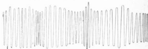
(C) FREQUENCY-MODULATED WAVE WITH AMPLITUDE AFFECTED BY INTERFERENCE
