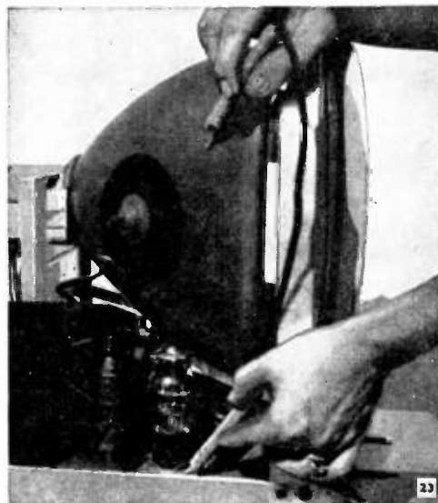
Shorting picture-tube coating to chassis
