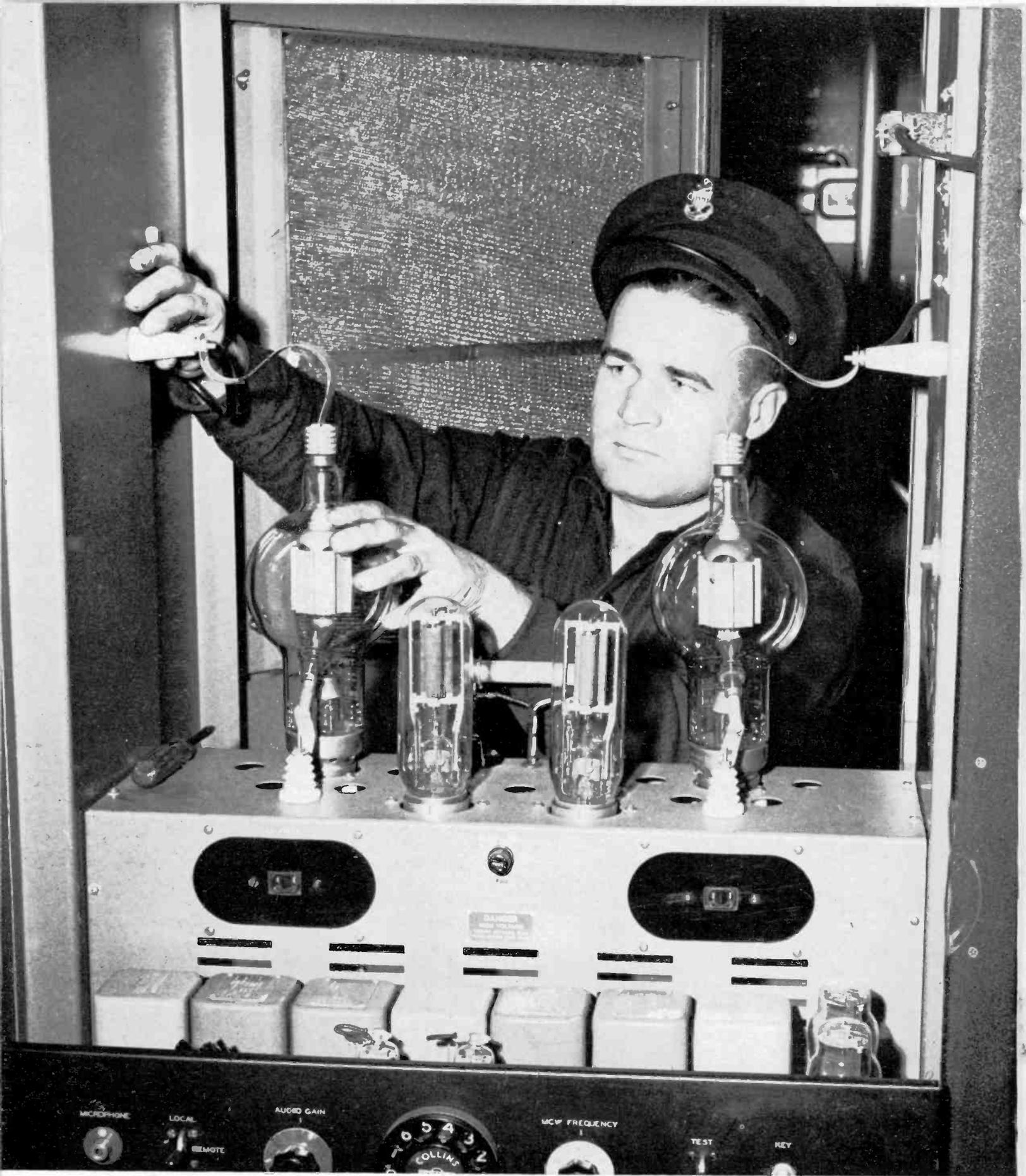
The USCG cutters' communication transmitters are Collins three-kilowatt 231D models. Autotune controlled, these transmitters are used as ship-
