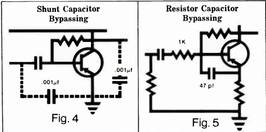
Leads should be kept as short as possible especially with bypass capacitors. The lead length determines the resonant frequency, and therefore, the effectiveness of bypassing. Bypassing directly to the emitter is often more effective.
