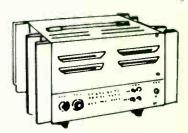
MODEL A51 High quality stereo power amplifier. output 25+25 watts rms into 8 or 15 ohms. Distortion under 0.05%. Power and frequency response ± 0.5dB 10-20,000 Hz. Size 131/2 x 81/2 x 10".
