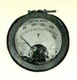
500 microamp. panel meter with luminous markings. Requires 21/6" dia. Hole for clamp (supplied) fixing. Resistance 500 ohms. moving coil.
