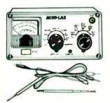
A multi-function and multi-purpose Ten-in-One tester. It combines its innate performance as a tester with functions of field strength indicator, generator, resistor, condenser and battery supply. The Mini-Lab, in its small case, is completely battery operated and suited for quick checkups in service shops and home-service calls.
