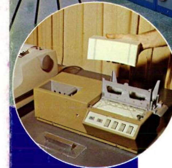
Top photo shows IGM 600 control system with card reader and typewriter rack-mounted. Inset shows optional remote positioning of card reader and typewriter in separate desk console.
