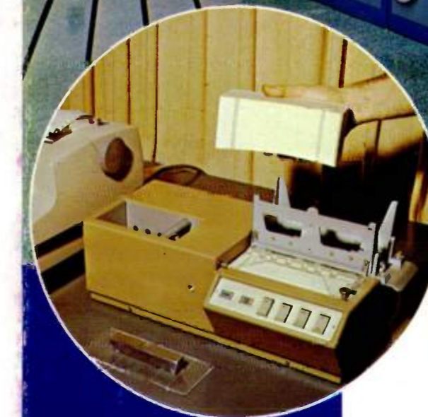
Top photo shows IGM 600 control system with card reader and typewriter rack-mounted. Inset shows optional remote positioning of card reader and typewriter in separate desk console.
