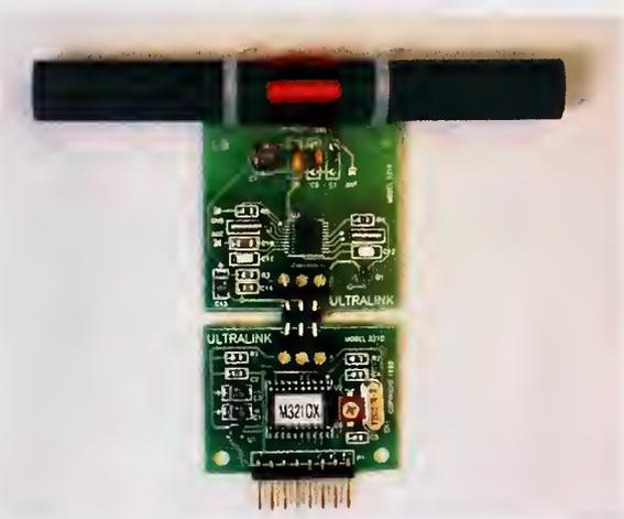
Figure 2.9. WWVB Receiver Circuit
