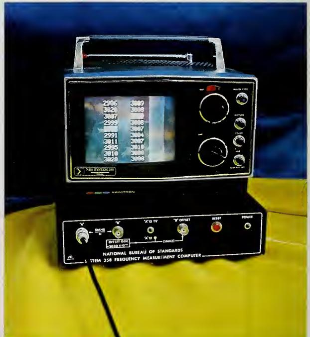
Figure 8. Prototype of a digital offset computer.
