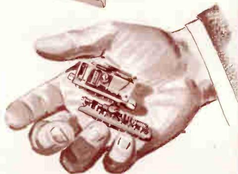
*The Tuner Strips shown here are similar to those already on the Station Selector—except that they have been designed to tune to an Ultra High Frequency Channel. They are simply snapped into place, and one screw adjusted for perfect reception of picture and sound.*
