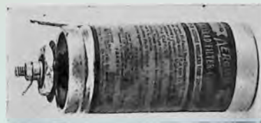
A dry-electrolytic 100 microfarad bias-bypass.
