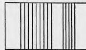
Fig. 1. "Spinning" turns to adjust a coil.
