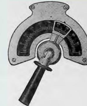
the shaft of the tuning unit. A scale and a blank calibration arc with a second indicator are provided.
