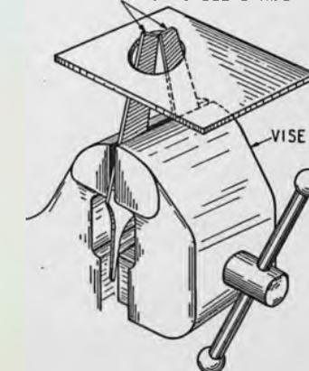
A reamer for meter-holes in aluminum and insulating panels.
