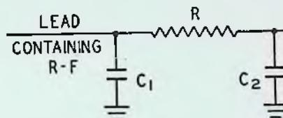
Fig. 1. The resistance-capacity filter. At radio frequencies the parts have the values given in the text for '24 plate circuits or screen circuits. Where a c-bias lead is to be filtered the condensers remain unchanged but the resistor is 100,000 ohms. For audio work 1 microfarad condensers are useful but even .01 is made useful.
