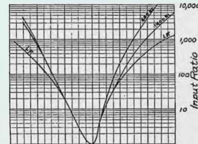
Selectivity curves. The curves are shown in the usual manner, the lowest point being at resonance and the two extremes 30 kc. off to either side. The height of the curve indicates the ratio in which input must be increased to maintain the same output which was obtained at resonance. This is, of course, an indication of the degree of discrimination against unwanted signals.
