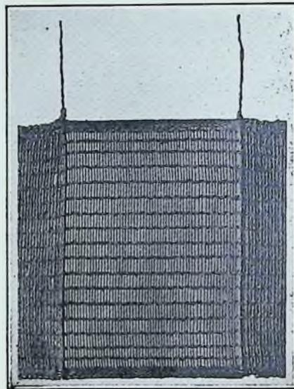
An "Ohmspun" resistor suitable as an r.f. load. Asbestos thread is the warp, resistance wire the woof. The inductance and distributed capacity are low, the aircooling good. The units come in values from 46 to 1000 ohms. The lower-resistance ones will dissipate about 1/4 kw. while those above 230 ohms will dissipate 100 watts each. Tapped Units are available as are racked series and parallel groups. Makers, The States Co., New Park Ave., Hartford, Conn.
