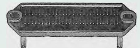
A "Plaque" resistor suitable for high frequency work. A resistance wire is wound in a sort of progressive figure 8 form and then laid into a miniature porcelain trough and sealed with vitrified enamel in the usual Ward Leonard manner. Rating 40 watts, obtainable tapped or untapped 100 or 5000 ohms. Makers, Ward Leonard Electric Co., Mount Vernon, N. Y.
