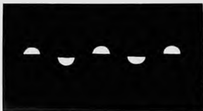
End view of a neon lamp crossing a dark room in a hurry, just to prove that the plates light alternately as shown in the next figure.
