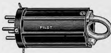
Two kinds of good coil forms, illustrated by the National, one of R-39 low-loss material and Pilot's bakelite form ribbed to keep the wire away from the bakelite.
