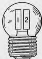
One type of neon lamp which may be used as an indicator. Plate 1 lights on the positive half of the cycle. Plate 2 lights on the negative half of the cycle. See also photo at head of this paper.
