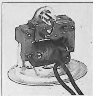
A synchronous clock-motor equipped with the necessary mirrors as was explained in the February issue.
