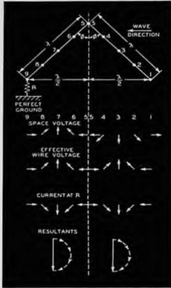
Fig. 4. The V-shaped antenna provides an array of two tilted wires which not only reinforce each other but leave the optimum direction of response unaltered over a considerable range of frequencies.
