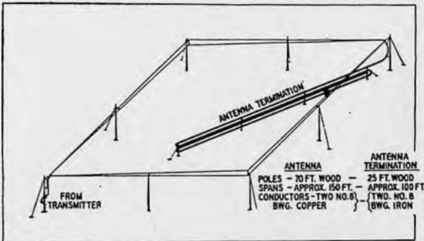
Fig. 9. For transmitting antennas, a terminating impedance of the required dissipating ability has been found in a long two-wire transmission line shorted at the far end. See note at the end of this paper.
