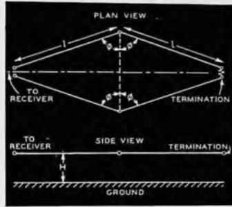
Fig. 8. When one V balances another in a diamond-shaped array, the terminating impedance need not be grounded but can be connected between the far ends of the two V's.
