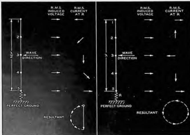
Fig. 1. The voltages induced by a horizontally propagated wave in a vertical half-wave antenna (left) are all in phase. On reaching the receiver, the resulting currents are out of phase: the vector resultant is the diameter of a half-traced circle. For a full-wavelength antenna (rear, left), summing the vectors traces a complete circle, and the resultant is zero.
