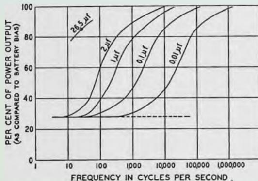
Fig. 4. Unless one uses push-pull, or a circuit like Fig. 5, it is necessary to use high-capacity bypasses on audio cathode resistors. The common ½ to 1 mike is absurd—unless one has a poor filter and must get rid of hum and bass together!
