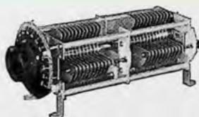
Split-stator type. For medium power push-pull transmitters and "High C" Circuits. Especially suited for five meter work. Isolantite insulation. Polished plates with rounded edges. Special bearings, rigid frame. For 3000 and 6000 volts.
