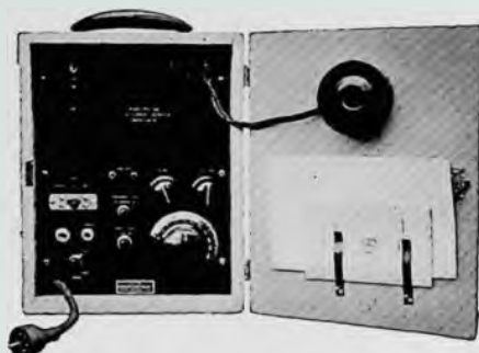
The C. W. and phone transmitter and receiver. Microphone on set cover with cord plugged into pinjacks, and additional jack and transformer tap providing for plugging in a phone line for remote pickup. The receiver tuning controls are at lower right, filament switches and meter jack at center and sending controls at left. At the top an antenna lamp, next a send-receive switch, then jacks for headset and key, a 2-point power-level switch and finally the cord and plug to connect to the battery box.
