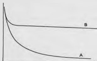
Fig. 1. Poor regulation of an ordinary high-vacuum diode rectifier (A) and comparative performance of mercury-vapor type (B).
