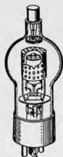
Fig. 2. A General Electric thyatron. Some thyatrions can be used as inverters.
