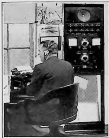
Fig. 4. A commercial rack-type installation. From the top down—Permanent-magnet dynamic speaker, coils storage rack, AGS receiver for traffic work, 58C tuned r.f. receiver for standby work, and the double powerpack for both.
