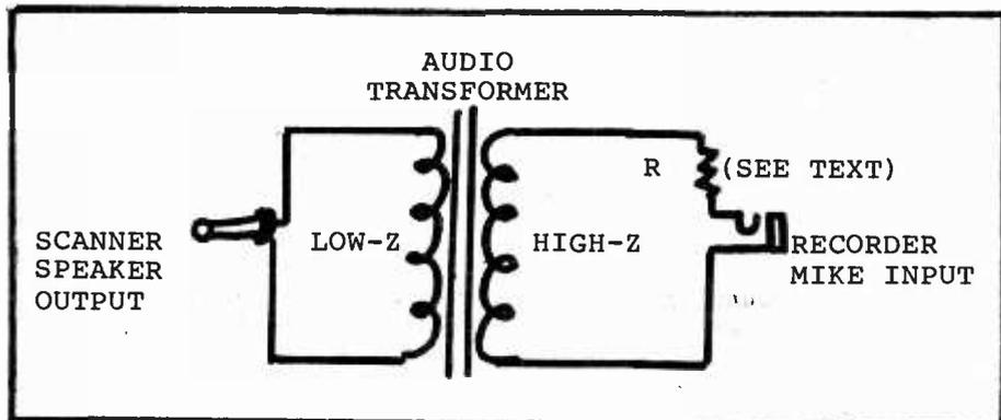
Schematic diagram of recorder coupler
