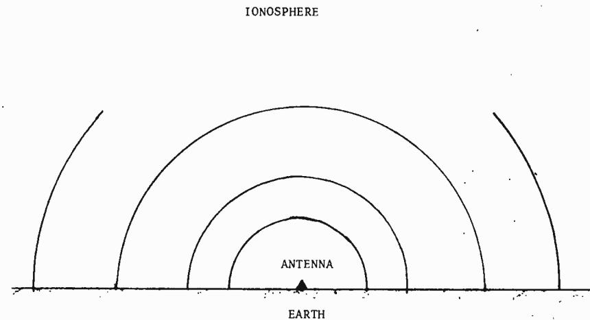
This figure illustrates that as distance from an antenna increases to many wavelengths, the wavefronts change from spherical to planar in shape. In many calculations, considerations are simplified with plane waves. Unfortunately, with terrestrial ELF propagation we are never very many wavelengths away and so have more complex problems.
