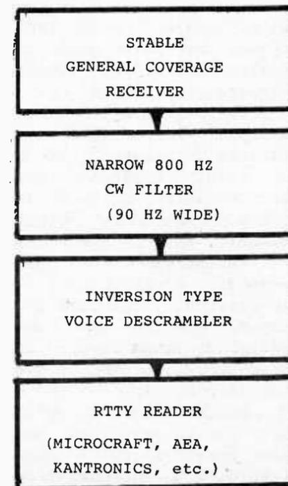
The CW filter selects the discrete channel desired, while the inversion-type voice descrambler, commonly available to scanner listeners, is tuned to convert the tones from the sharp CW filter (approximately 800 Hz) back to tones near 2 kHz for the RTTY reader or demodulator.
