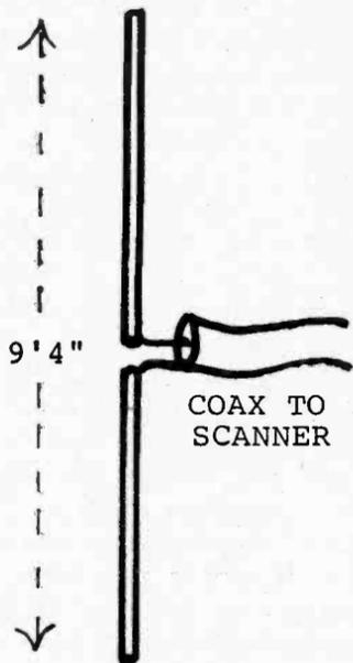
Experimental antenna for scanners
