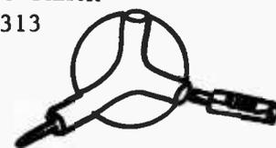
COIL MOUNTED IN MOTOROLA PLUG
