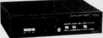
**SWL-TEXT is the software and CP-1 is the interface that when combined with your Commodore C64™ and communications receiver, will give you everything you could ask for in a CW/RTTY intercept station!**
