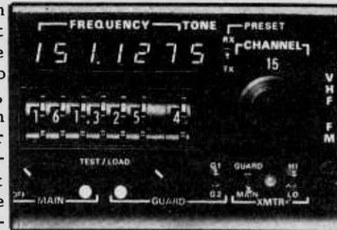
*The Wulfsberg Programmable transceiver covers all VHF channels from 138 to 174 MHz.*
