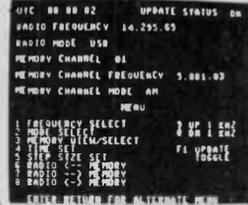
**MAIN MENU** Control center for entire system. Showing 24HR UTC time, radio freq. & mode, memory CH, freq. mode plus ID functions for your selection.
