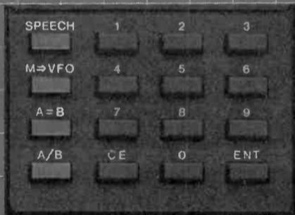
**Keyboard Entry.** ICOM introduces a unique feature to shortwave receivers...direct keyboard entry for simplified operation. Precise frequencies can be easily selected by pushing the digit keys in sequence of frequency. The frequency will be automatically entered without changing the main tuning control.
