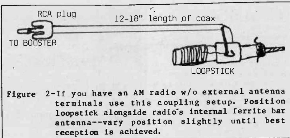
Figure 2-If you have an AM radio w/o external antenna terminals use this coupling setup. Position loopstick alongside radio's internal ferrite bar antenna--vary position slightly until best reception is achieved.
