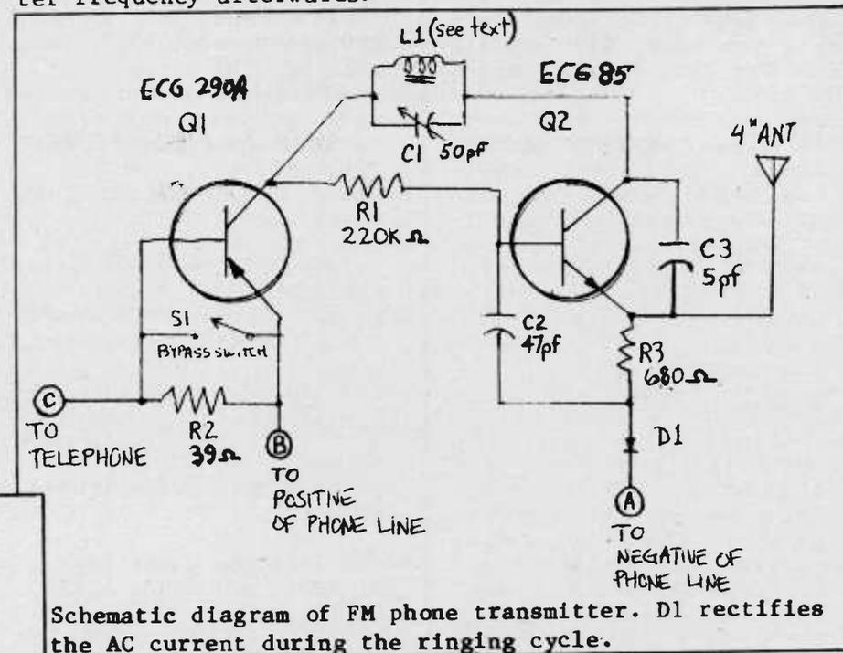
Schematic diagram of FM phone transmitter. D1 rectifies the AC current during the ringing cycle.
