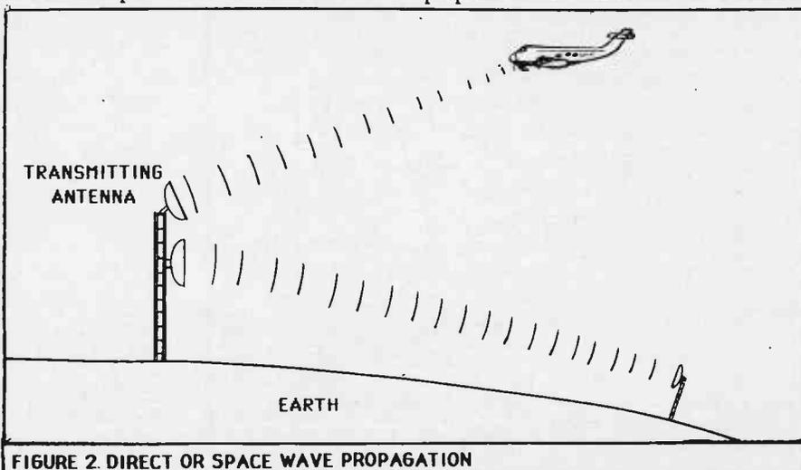
FIGURE 2. DIRECT OR SPACE WAVE PROPAGATION
