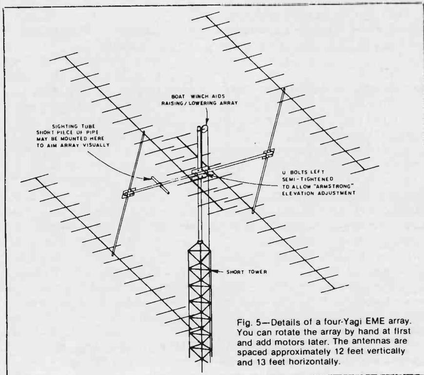
Fig. 5—Details of a four-Yagi EME array. You can rotate the array by hand at first and add motors later. The antennas are spaced approximately 12 feet vertically and 13 feet horizontally.
