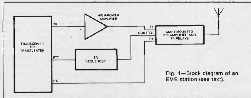
Fig. 1—Block diagram of an EME station (see text).
