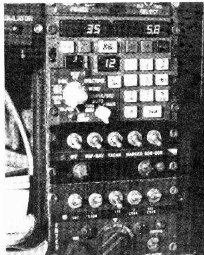
Navigator's crew position radio console (lower half of panel) on KC-135 showing toggle switches to select which radios/intercom to hear and transmission selector knob.
