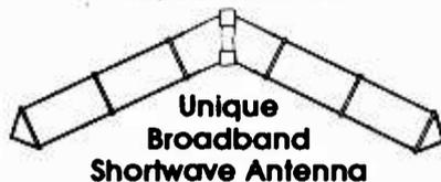
Utilizing the same principles as the B & W world-acclaimed transmitting antennas, this patented receiving antenna provides outstanding coverage of all the frequencies in the shortwave region. With coaxial cable feed, the SWR is less than 2:1 throughout the 3.5 to 30 MHz spectrum. Good MW and LW reception is also provided by this big antenna. Rugged construction with #14 stranded copperweld wire. SC-239 connector for coaxial cable. Only 90 feet long.
