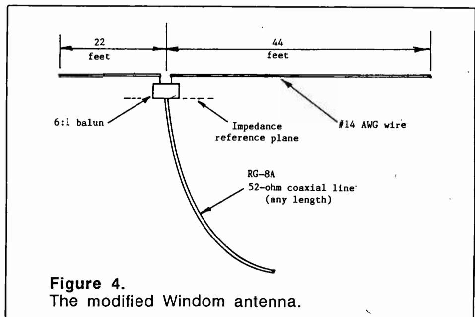
**Figure 4.** The modified Windom antenna.
