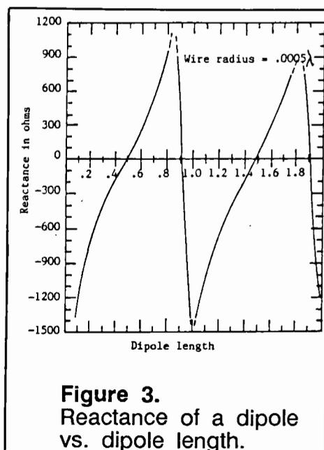
**Figure 3.** Reactance of a dipole vs. dipole length.
