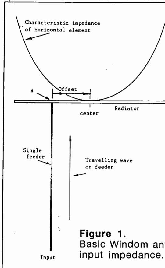
**Figure 1.** Basic Windom antenna. Impedance at point A must equal input impedance.
