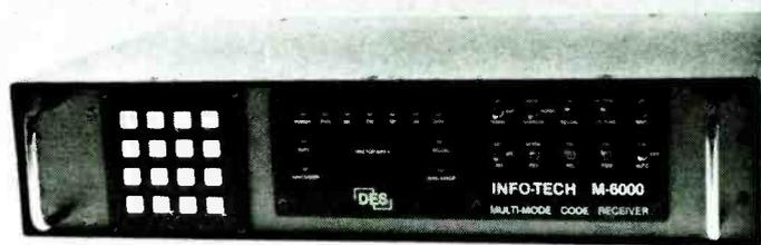
Additional LED status lights assist proper adjustment, as well as displaying accurate band readout.
