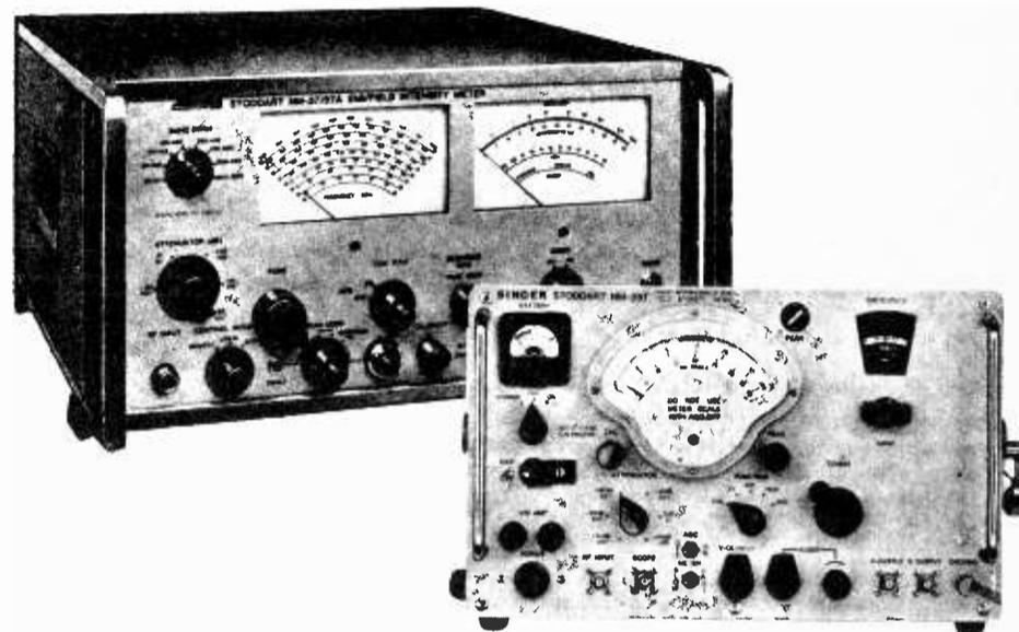
Popular among VLF listeners are commercial or military surplus frequency selective voltmeters like the Rycom R2174 and noise measuring test sets like the Ailtech NM17/27A and Singer NM25T shown here.
