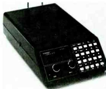
The Regency TS-2 boasts the fastest scan and search rates in the industry—50 channels per second—more than three times faster than the next closest competitor. Six memory banks store up to 75 separate frequencies, selectable by groups or in a continuous sequence.
