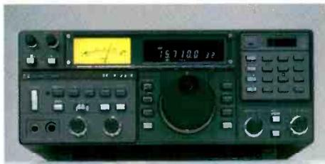
**The IC-R71A** is a shortwave listener's delight. Its 32 tunable memories store frequency and mode information, and they are single-button reprogrammable independent of VFO A or VFO B's operations! This HF reception is further enhanced by a dual width and level adjustable noise blanker, panel selectable RF preamp, selectable AGC, four scan modes, and all-mode squelch.
