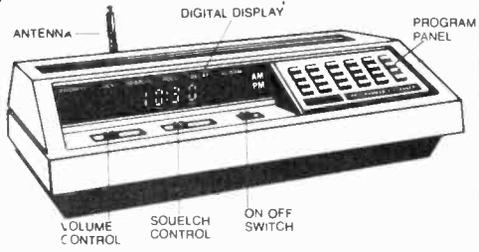
The Regency Z30 is a compact, programmable 30 channel, multi band, FM monitor receiver for use at home or on the road. It is double conversion, super heterodyne used to receive the narrow band FM communications in the amateur, public safety and business bands: 30-50, 144-174, and 440-512 MHz. Size 10 3/4"Wx2-7/8"Hx8-3/8"D.
