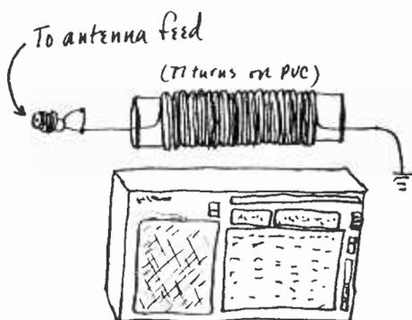
The signal from the Caribbean Beacon on 1610 kHz is boosted as the coil around the PVC pipe is brought nearer to the receiver's internal ferrite rod antenna.
