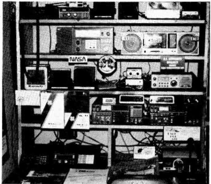
*Bill Battles' (E.Kingston, MA) well-equipped monitoring post: ICOM R-70 and R-71A, Realistic DX-400 receivers; Realistic PRO-2004, Regency MX3000, Regency ACT-R-106 scanners; Unimetrics SSB CB; ICOM M-80 VHF scanning marine txvr; Sonar VHF-Txvr. Nice set-up, Bill!*
