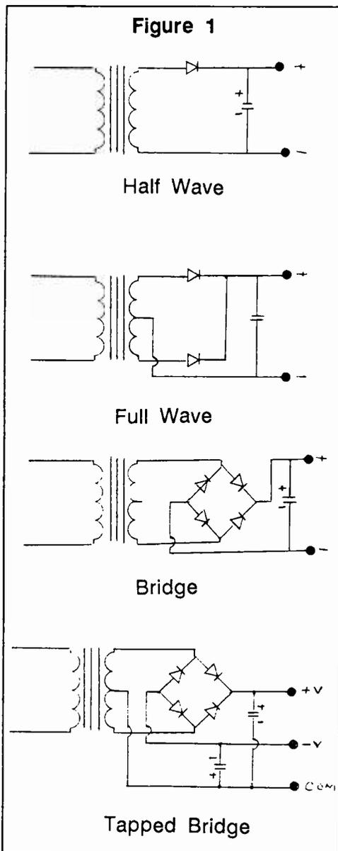
various common power supply circuits and regulators, along with the information on getting the output you need with the parts on hand. As we go along, I'll try to point out some pitfalls and fine points that can make the difference between power and fire.
