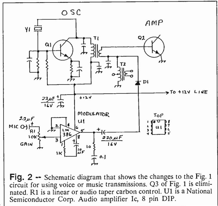
**Fig. 2** -- Schematic diagram that shows the changes to the Fig. 1 circuit for using voice or music transmissions. Q3 of Fig. 1 is eliminated. R1 is a linear or audio taper carbon control. U1 is a National Semiconductor Corp. Audio amplifier IC, 8 pin DIP.
