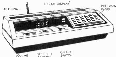
The Regency Z-60 is a compact, programmable 60 channel, multi band, FM monitor receiver for use at home or on the road. It is double conversion, super heterodyne used to receive the narrow band FM communications in the amateur, public safety and business bands. 30-50, 118-136, 144-174, and 440-512 MHz. Size 10 3/4" Wx2 7/8" Hx3 3/8" D.
