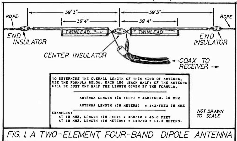
FIG. 1. A TWO-ELEMENT, FOUR-BAND DIPOLE ANTENNA
