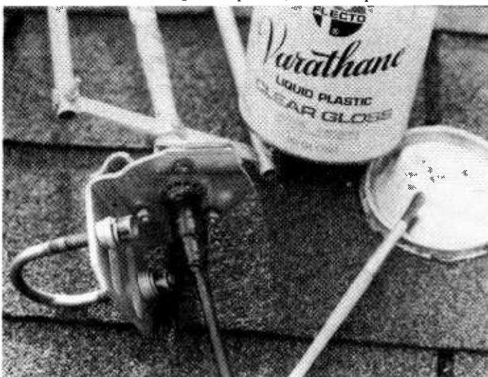
*One top ten scanning secret: To lock out moisture, wrap your antenna connection with electrical tape and brush on a coat or two of urethane.*
