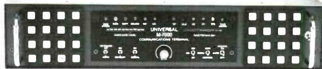
Plugs into your receiver's speaker or earphone jack to provide a printout of messages sent in Morse code (5-120 WPM), Moore code, RTTY (45-250 baud), ASCII (75-1200 baud), TOR (FEC and 2/4 channel, 86-200 baud ARQ), packet, TDM, FDM (4 channel), Russian Cyrillic (video) as well as FAX photos (3 IOCs)!
