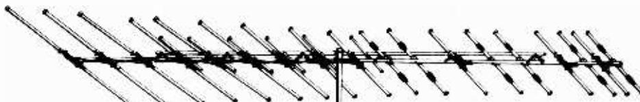
*A high gain VHF antenna may make use of both log-periodic and Yagi beam principles.*
