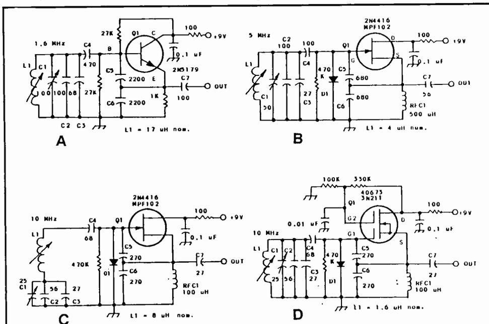
**Fig 1** - Schematic diagrams of four versions of the Colpitts oscillator. Circuits A, B and D are parallel tuned. Circuit C is series tuned. Compare C to D to learn how the L1 inductance changes when using a series-tuned circuit. All other component values remain the same, as does the operating frequency (see text).
