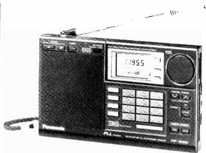
FM/LW/SW) mini-portable, boasting 36-station preset, keypad, rotary, up/down manual, scanner and meter band direct access tuning.
