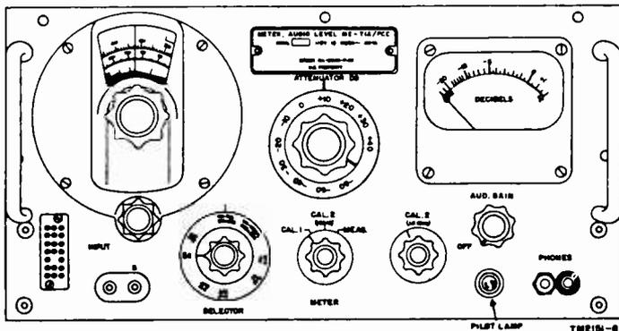
**Fig. 1 - Audio Level Meter ME-71A/FCC**
