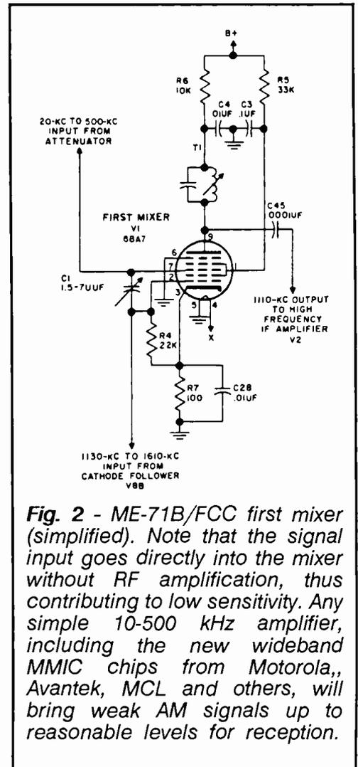
**Fig. 2 - ME-71B/FCC first mixer (simplified).** Note that the signal input goes directly into the mixer without RF amplification, thus contributing to low sensitivity. Any simple 10-500 kHz amplifier, including the new wideband MMIC chips from Motorola, Avantek, MCL and others, will bring weak AM signals up to reasonable levels for reception.
