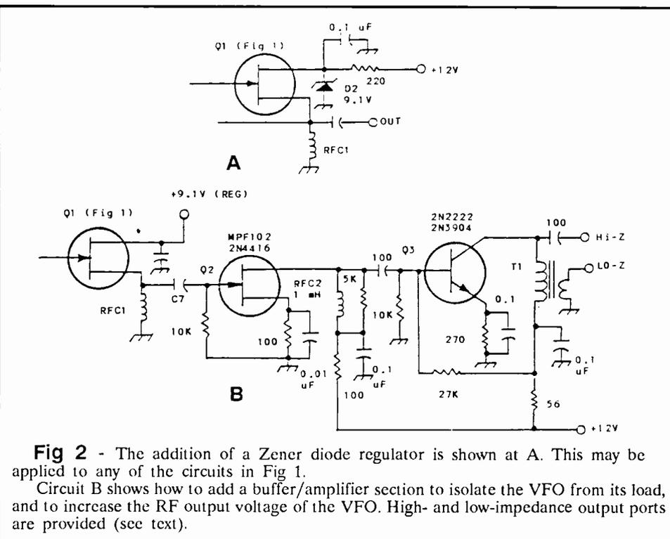
**Fig 2** - The addition of a Zener diode regulator is shown at A. This may be applied to any of the circuits in Fig 1. Circuit B shows how to add a buffer/amplifier section to isolate the VFO from its load, and to increase the RF output voltage of the VFO. High- and low-impedance output ports are provided (see text).
