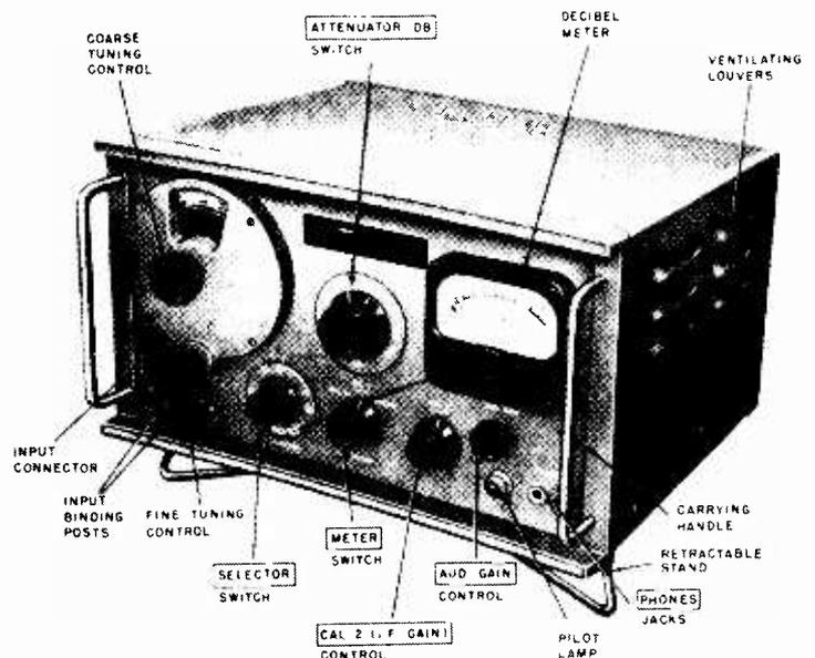
No internal speaker is provided, but a front-panel headphone jack is convenient for direct monitoring of amplitude modulated signals such as non-directional beacons (NDBs) which still populate this portion of the spectrum.
