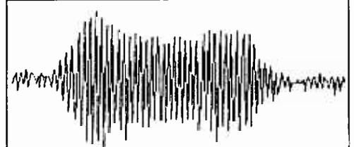
Fig 1: A single "Mark" tone from 850 Hz shift RTTY copied on 10.500 MHz (M7000 scope output), displayed on a Tandy 1000TL
