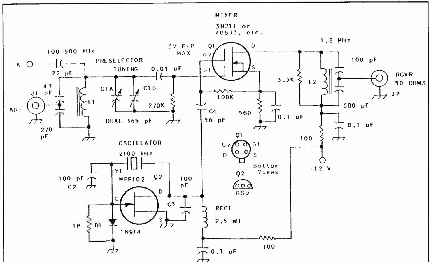
**Figure 1** -- Schematic diagram of a practical LF/VLF converter that can be used with a general-coverage receiver. Resistors are 1/4-W carbon composition. Fixed-value capacitors are disc ceramic, 50 V rating or greater.
