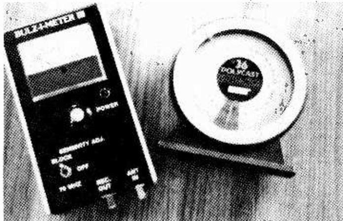
*With the Bulz-I-Meter, an inclinometer, and a couple of wrenches, you can peak the sparklies right off your screen!*
