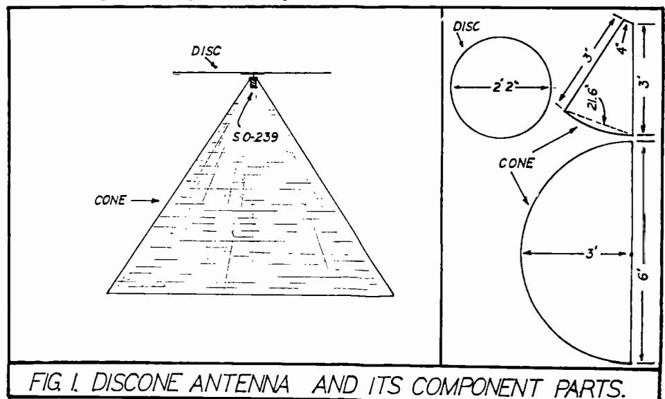
FIG. 1. DISCONE ANTENNA AND ITS COMPONENT PARTS.
