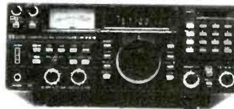
**R7000**-There is nothing to compare with the R7000 under \$12,000. This is the most sophisticated V/UHF receiver ever offered to the public. No wonder it's our best selling V/UHF receiver. All mode AM, SSB, CW, FM, FMN-25 to 2000 MHz (20 kHz to 2 GHz w/NOVEX FC7100), direct keyboard entry. 99 memory channels, many ICOM options plus EEB options and high performance package deal. (CALL)
