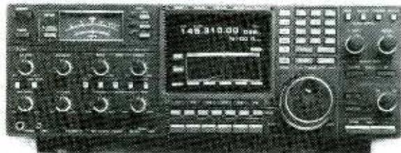
The incredible Icom R-9000 receiver features continuous all-mode coverage from .1 to 1999.8 MHz. The ultimate in sophisticated monitoring is achieved with a built-in multi-function CRT that displays spectrum use, memory configurations, timers, and more. Seven types of scanning and 1000 memories are provided.
