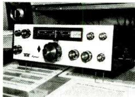
Fig 6: Here's the finished product. A highly modified Argonaut 509 that will hold its own in a contest or ragchewing on 40 meters.
