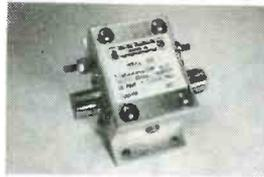
Unlike any other lightning protection device for coaxial transmission lines, I.C.E.'s Model 300 series requires no predetermined voltage to develop between conductors before voltage suppression begins. Units are constant drain, capacitor-blocked, non-DC passive, and each relies on a heavy discharge inductor paralleled with a ceramic gas-discharge assembly to provide a lightning-fast trap system for induced voltages.
