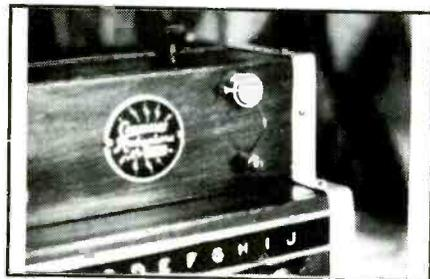
Detail of the "cat's whisker" and galena crystal assembly. One spent quite a good deal of time hunting around on the surface of the crystal for the "hot spot."
