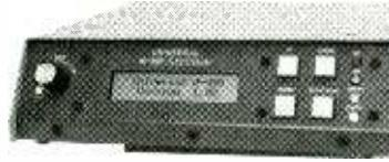
The display is a two-line LCD, 20 characters (5/7 dot matrix) per line. A low pass filter at 1275 Hz mark frequency permits shifts of 170, 425, 850 Hz and variable 100-1000 Hz.
