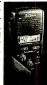
**Very warm but not quite hot:** Radio Shack's new TR-493 mobile radio with digital signal processing helps to take some of the high-pitched noise out of CB communications at the flip of a switch, but at a hefty price. Unfortunately, the more stubborn pulse-type noises are untouched. This is an interesting concept that holds great promise for future development.
