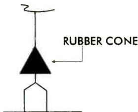
Several readers reported poor antenna performance as a direct result of ice build-up between the vertical element and metal base. The problem was corrected by utilizing a rubber cone (sketch at left). Similar to an umbrella, the cone prevented ice from grounding the vertical element to the antenna base.
