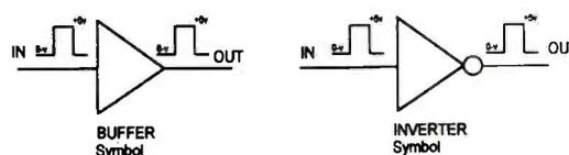
BUFFERS and INVERTERS are the simplest of all. First, both are properly called "buffers" with specific terms to identify each type: non-inverting buffers and inverting buffers. I shall refer to them as "buffers" and
