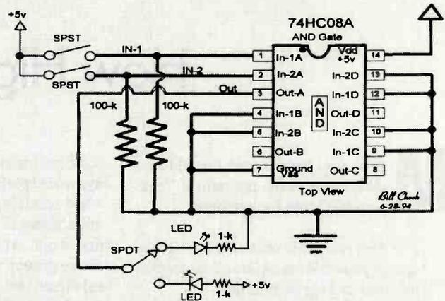
*Note: Bold traces are the required AND circuit. Light traces are the optional control interface. The SPST switches can be a simple 2-seg DIP switch. The SPDT toggle switch and LEDs demonstrate the two different ways to derive logical outputs for this type of AND gate. Eliminate the light-trace circuits and add your own In/Out requirements as desired.*
