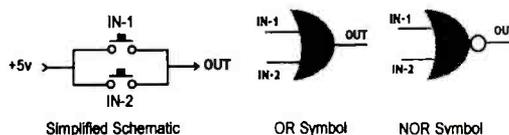
Next, we have the OR gate. Either switch closed (or both: it doesn't matter), will produce an output high. An OR gate could be used to trigger an alarm if either smoke OR heat existed, see? The opposite logic of the OR is the NOR and like the NAND, it is more difficult to depict than to describe. Neither an input on 1 nor an input on 2 are required to get an output high. Conversely, there is no output high if there is an input high on either 1 or 2 or both.
