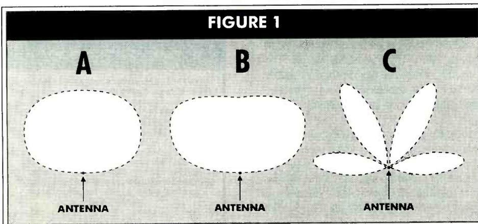
*Vertical directivity patterns for horizontal single-wire antennas viewed from one end of the antenna. Antenna height above electrical ground is (A) 1/4 wavelength, (B) 3/8 wavelength, and (C) 1 wavelength.*
