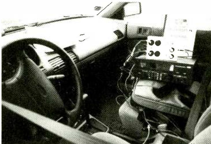
*Author's DX equipment includes a Drake R8, homebrewed dual antenna phaser (DCP-1), and remote controller.*
