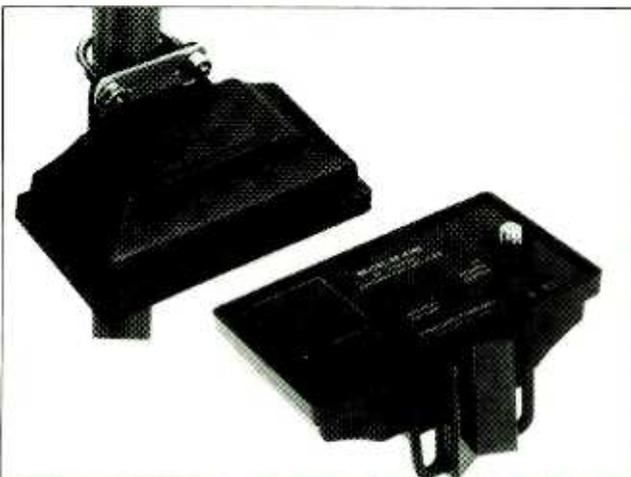
*Mast mounted preamplifier amplifies the antenna signal at the antenna before it goes down the feed line. This Chromstar model AP-8783 by Winegard provides 17 dB gain at VHF and 28 dB at UHF frequencies. (Courtesy Winegard)*
