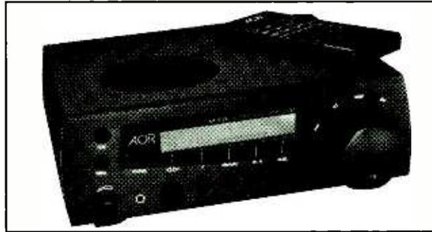
XX.XXX.XX MHz format, along with a wide variety of other visual information; passband tuning; a six-level attenuator (including preamp); an all-mode squelch; rear connectors for coaxial and wire antennas; and a switch for choosing between antennas, including a whip. Beady-eyed DXers will mourn the absence of a notch filter, but a tunable audio notch filter will be offered as an extra-cost option starting sometime late this year.
