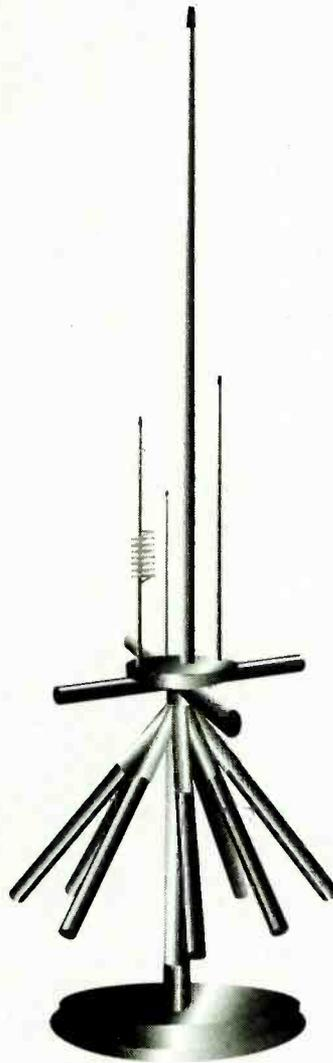
four horizontal elements are three-inch rubber ducks.
