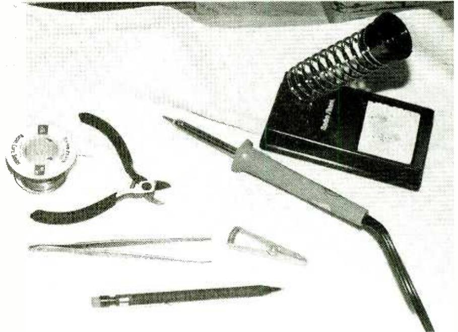
*My state-of-the-art tool kit: solder, soldering iron and holder, diagonal cutters, tweezers, and a pencil. Tapping joints with the eraser helped me find bad solder connections.*
