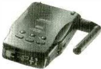
Uniden's Beartracker series is intended to provide easy access to public safety frequencies for the highway traveler. There is no frequency display, just a two-character LED to identify the state of choice and certain functional call-outs. Tiny and lightweight, the units can be attached to the windshield or dash by suction cups (provided) or to the sun visor. A short swivel antenna may be removed, exposing the BNC connector which allows attachment to a cartop antenna.
