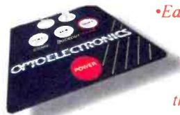
•Easy touch control pad. F1 & F2 keys control all Xplorer functions. Hold, Skip, Store and Lockout all enabled through the keypad.
