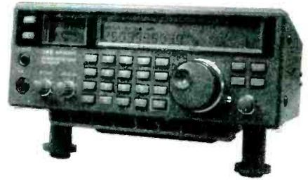
AOR has scooped the market with their new AR5000 extended-frequency coverage receiver, tunable from 10 kHz through 2600 MHz (less cellular) and offering 650 memory channels. For the first time, you can hear VLF time signals and naval communications, international shortwave broadcasting, worldwide single-sideband communications, civilian and military aeronautical transmissions, VHF/UHF public safety radio, ham repeaters, microwave earth satellites, and much, much more all on one receiver!
