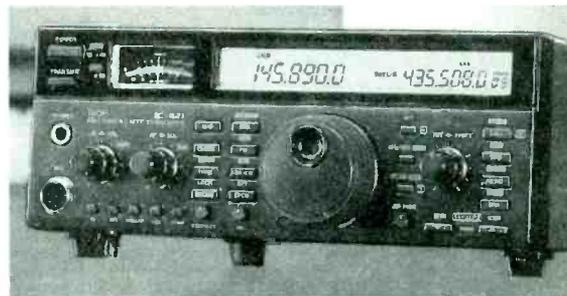
An all mode transceiver such as this ICOM IC-821H can get an amateur on all of the modes available to a Technician Class ham.
