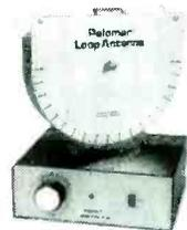
Loop amplifier gives 20 dB gain and sharp tuning. Plug-in loop Model BCB covers 540-1600 KHz AM band. Rotates and tilts to give best possible reception. Other plug-in loops cover 10 KHz to 5 MHz.
