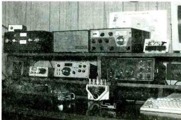
The current line-up at K7SZ, L-R from the top: Dentron MT3000A tuner, Drake MS-4 speaker, Drake TR4C HF SSB/CW transceiver. 2nd shelf: amplified speaker, Wilderness Radio Sierra, Ten-Tec Century-22 and Yaesu FT301D HF transceivers. The Ten-Tec 1208 6m is off camera. Note the Alpha Delta four-position RF switch which controls the antennas.
