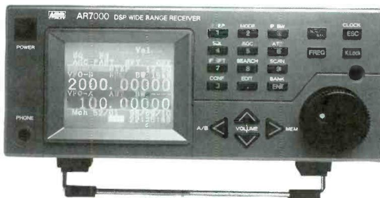
The 7000's characteristic 0.5 microvolt sensitivity (SSB and FM) captures even the weakest signals, while dual-VFO operation permits you to toggle between two frequencies for listening to duplex communications.
