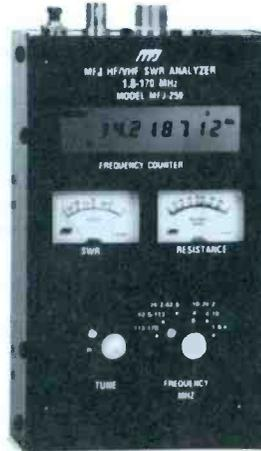
FIG. 1. The MFJ 259B SWR Analyzer
