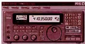
**FIG 1** - Main screen displays replica of IC-8500 front panel. You can use mouse buttons to activate radio controls.
