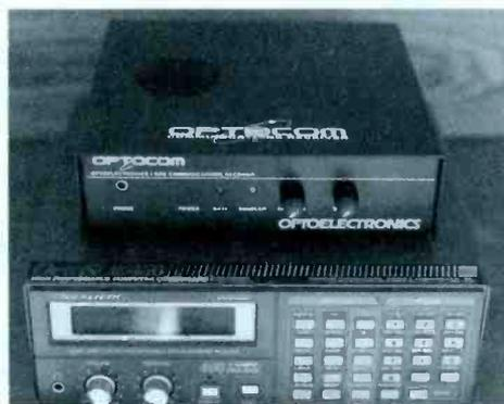
*The OS456 allowed computer control of the Realistic PRO-2006. Now, multiple-system trunk following and conventional scanning is available in a little black box.*
