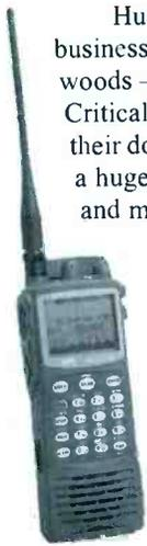
Grove Enterprises recommends the Alinco DJ-X10T or the AOR AR8200 handheld, wideband receivers for tracking these collar transmitters, which typically broadcast in the 169-216 MHz range. Up to 1000 frequencies can be entered, and the channels can be identified by collar number, name, color, etc. Depending on the terrain, reception can be expected from 2 to 3 miles.
