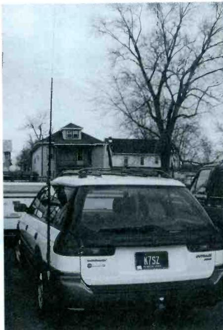
**FIG 1** - The Outbacker Outreach is affixed to the custom mount on my Subaru Outback SUV wagon. This rugged antenna is approx 9-ft long - "low profile" it ain't!
