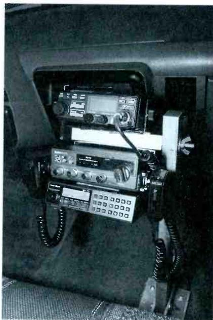
**FIG 4 -** My answer to a \$100+ commercial radio mounting system. This “Christmas Tree” mount is made from T-6061 aluminum bar stock. Notice that I have managed to hang three radios on the first cross piece. The 2 meter rig sits on top with a Radio Shack CB set underneath. Mounted to the bottom of the CB is a Radio Shack scanner. There will be a second cross piece added below the scanner to hold the GE Ranger-II 6 meter rig and a SGC-2020 HF transceiver.
