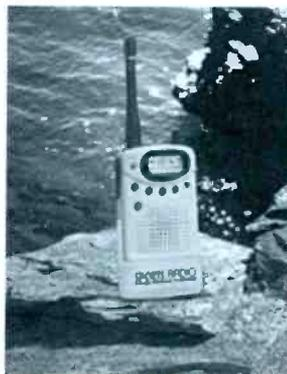
tially risky situations. An automatic polling function (called Vitalink™) that works with a pair of plusVWs allows a master unit to send out a 1-second polling transmission. The "slave" unit receives the signal and automatically transmits a silent response if it is within range. If not, an out-of-range indication is displayed on the master unit with an alert tone.
