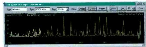
Click on a peak and you are instantly tuned. Alternatively, keep the left button down and drag your mouse across a scanned spectrum – you will see the frequency cursor moving, the frequency display updating accordingly and the receiver will be tuned following your hand movements!
