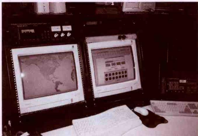
*From this high frequency direction-finding console, the FCC can remotely control its network of stations to locate signals from Hawaii to Puerto Rico.*
