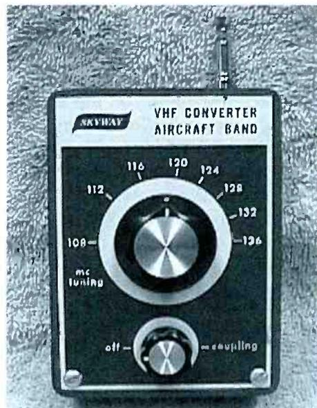
**FIG 2.** Old Skyway converter allowed VHF air band reception when placed next to a broadcast receiver (photo by R. Lucchesi, WA2RQY)
