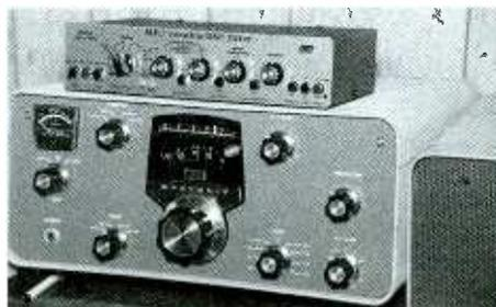
**FIG 2:** The MFJ 784-B DSP filter will add DSP to your existing receiver/transceiver at a fraction of a new radio with DSP built in. I use mine exclusively with my Heathkit SB-310 SW receiver.
