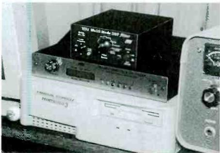
**FIG 3:** MFJ's 781 DSP unit is designed exclusively for multimode data controllers. My 781 is sitting atop the MFJ 1278-B MMDC, which is coupled to my Ten-Tec Argosy-II for HF packet, PACTOR and RTTY modes. A clean, noise-free signal is the key to HF data.
