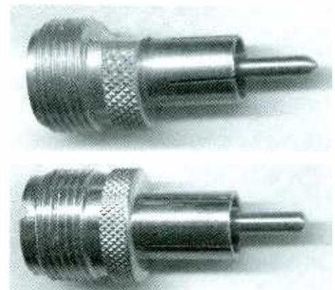
**FIGURE 2.** Female UHF to Motorola plug adaptor modified to fit BC248CLT (top). Unmodified adaptor (bottom)
